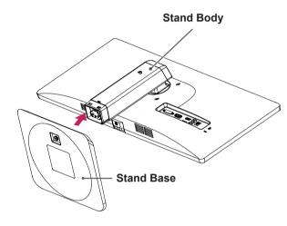
3 Using a coin, turn the screw clockwise to secure the **stand base**.
